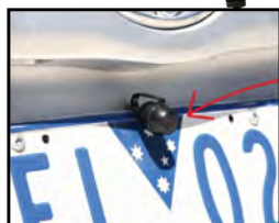
Mounting bracket sits behind the number plate and it is not visible.
